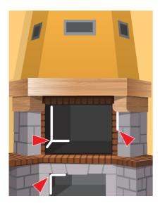
Tekadom 1200°C is a one-component fire resistant sealant made on the basis of inorganic silicates. It is used for repairing fire-places, stoves, chimneys and fire resistant brick
