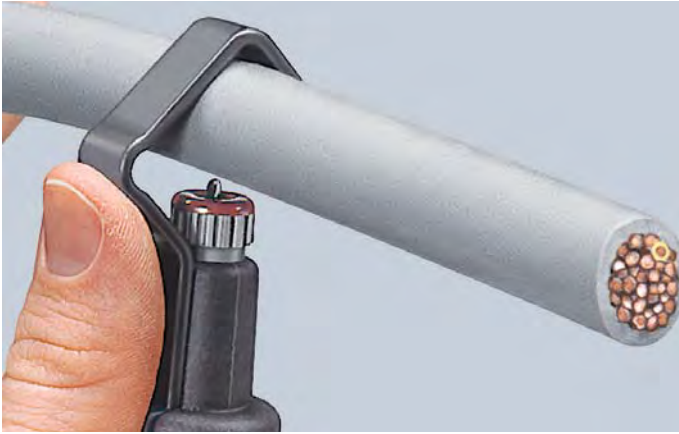
Setting the tool for circular cutting
