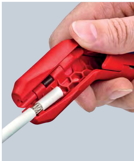
Dismantling of a coax cable
