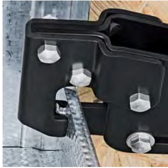
Setting the pliers for connection of two metal section sheets
