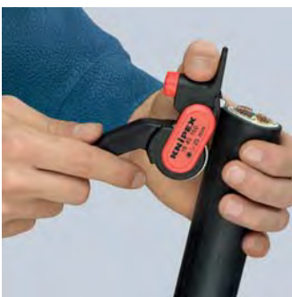
Setting the tool for longitudinal cut
