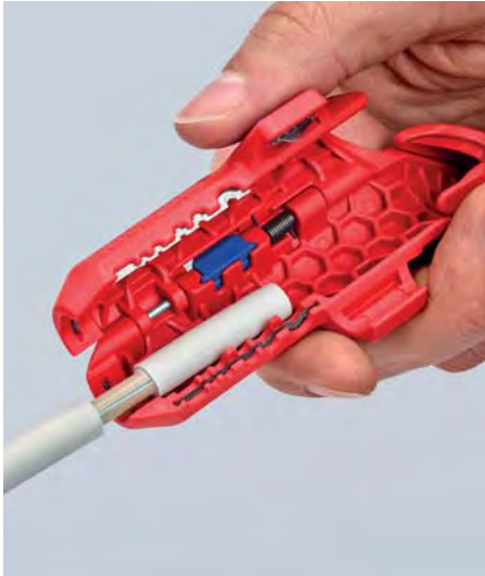
Dismantling of a NYM cable
