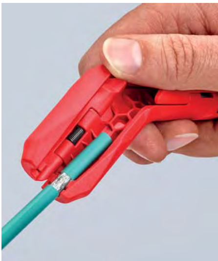
Dismantling of a data cable
