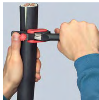
Turning the tool for circumferential cut
