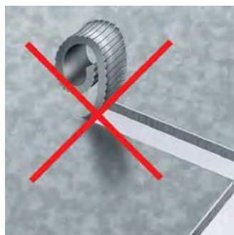
Notching without chip breaking
