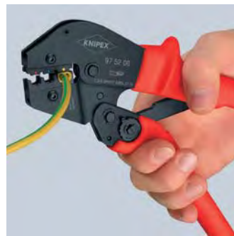
Second step: now use the whole hand for further crimping procedure
