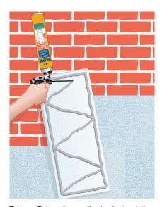
Tekapur Polyurethane adhesive for insulation plates is a low-expanding, one component polyurethane foam, suitable for fastening insulation materials with the help of a gun for PU foam. The foam hardens due to air humidity.
